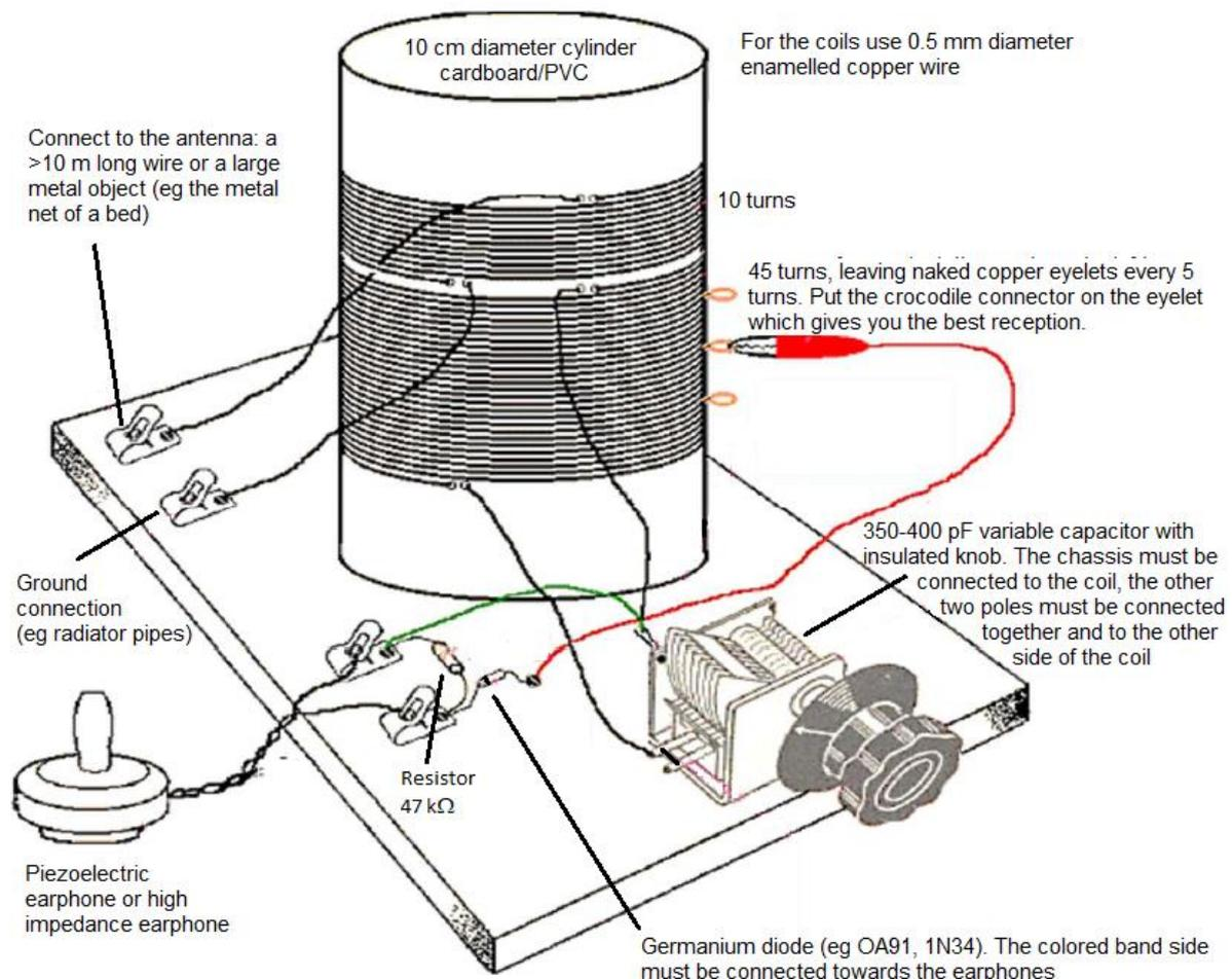
**An alternative with no antenna and ground connection:** On a square support of 50-60 cm side length (even a extra large pizza box could be ok) create two windings, one of 4 turns the other of 12 turns. The first winding must be connected to the diode, resistor and earphones, the other one must be connected to the variable capacitor. In this crystal radio the windings are so large that directly collect the radio waves.
